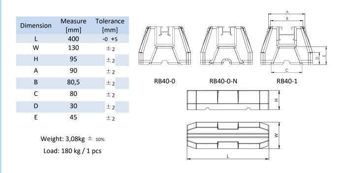
All products Fame Foot must in fact be installed according to the manufacturer's roof systems. The manufacturer of PVC membranes should advise on tendency to migration of plasticizers and define specific recommendations that should be taken into account during installation and which will guarantee that the roof is not affected.
